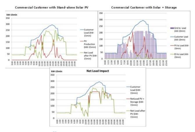
Figure 73 Output and net load impact of forecasted and modeled technologies
