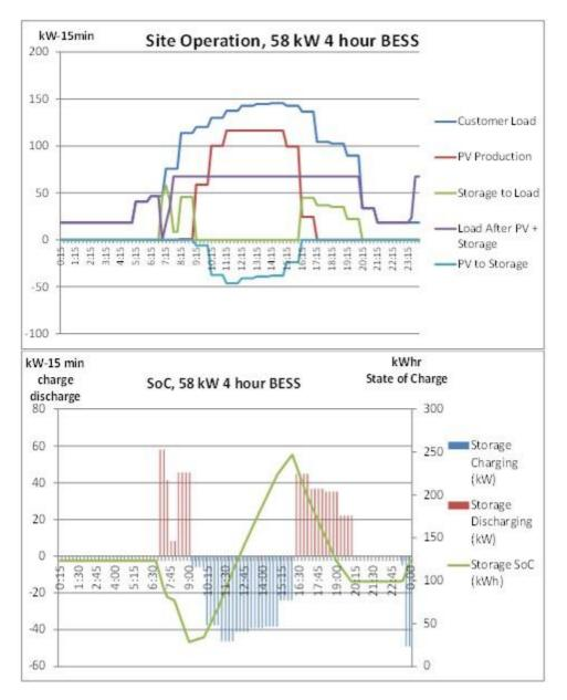
Figure 74 Example of Site and BESS operation at a small commercial facility
