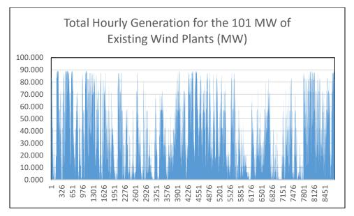
Figure 49: Total hourly wind generation for 101 MW existing wind plants
