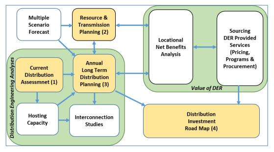
Figure 60 Integrated Distribution Planning Process
